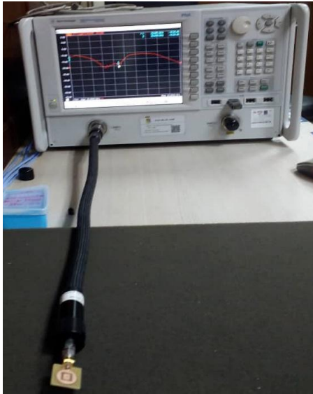
Figure 12: PNA measurement scenario
