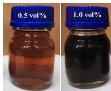
Fig. 5. Images of AgNPs–water NFs at different concentrations.
