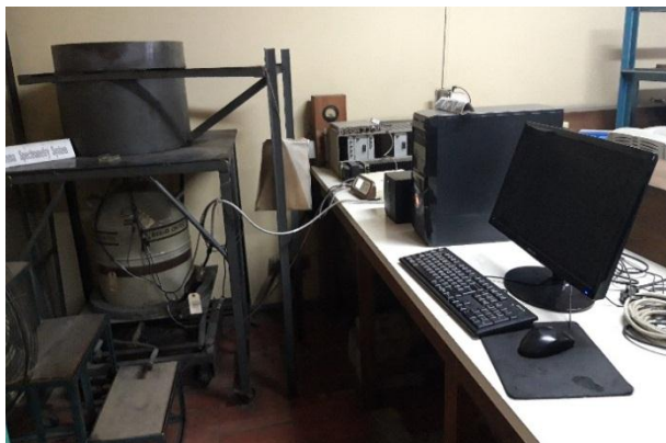
Figure 2. Photograph of laboratory setup for radioactivity measurement.
