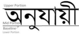
Fig. 3: Sections for a line-segmented image are shown. The “baseline” distinguishes between the characters and the modifiers below the characters; The “upper portion” is the upper slice that is divided by the headline or matra ; The “mid portion” is the area between the matra/headline and baseline. The “lower portion” is the area that lies below the baseline.
